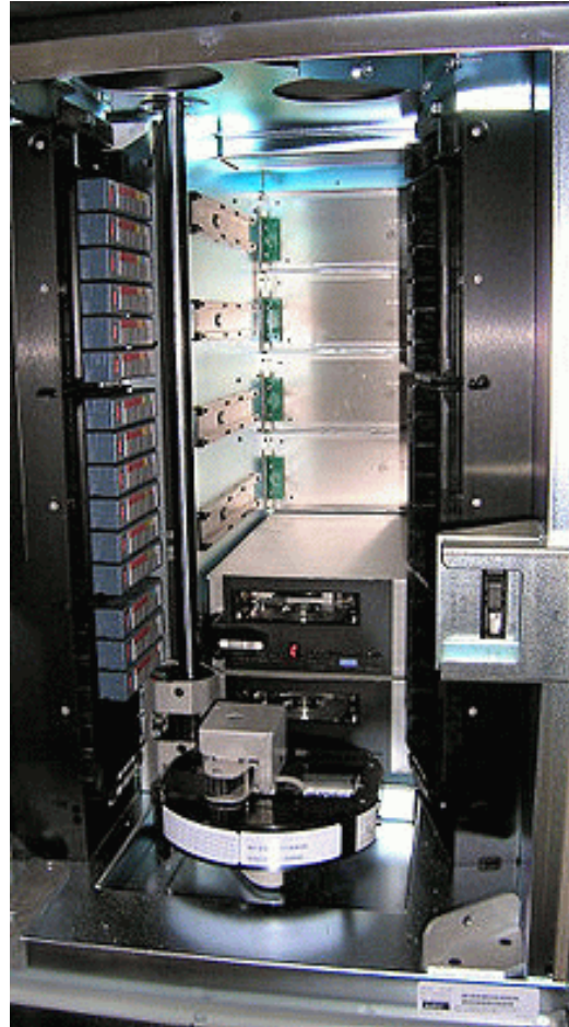
Small ADIC Scalar 100 tape library, robot visible on the bottom, two IBM LTO2 tape drives behind it.
