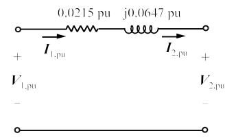
(b.) For a load which is 75% of rated value at a power factor of 0.6 lagging ( $\theta_v$  –  $\theta_i$  = 53.13°), the per-unit values of the voltage  $V_{2,pu}$  and the current  $I_{2,pu}$  are (using the voltage  $V_{2,pu}$  as the phase reference)
