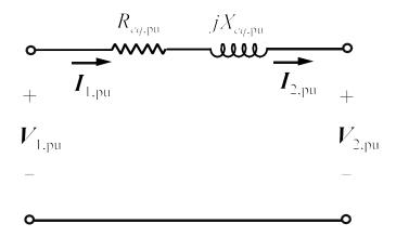
Note that there are no primed quantities in the per-unit equivalent circuit. Thus, there is no need to reflect impedances when using this model. Using the per-unit transformer model eliminates the need to scale quantities by the transformer turns ratio, thus eliminating a common source for error.
