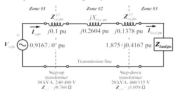
$$I_{load,pu} = \frac{0.9167 \angle 0^o}{1.875 + j(0.10 + 0.2604 + 0.1378 + 0.4167)} pu$$
